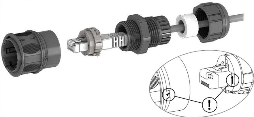
**Important:** Pay careful attention when inserting the grey cable sleeve assembly into the housing. Ensure that the parts are aligned exactly as detailed in the image above. Insert the grey sleeve and patch cable assembly into the housing until there is an audible click as it locks in place. If the grey sleeve assembly is incorrectly inserted, the IP67 Plug Housing cannot be connected to an EN-10.
